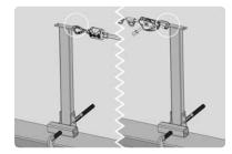
Identify suitable end anchors. This includes stanchions, heavy duty D-rings, suitably drilled I-beams, anchor slings, etc.
