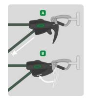
5. Pull excess line through tensioner [A] and close release handle [B].
