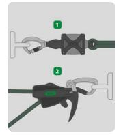
Connect the energy absorber end of the lifeline to anchorage point [1], and then connect the tensioner to anchorage point [2].
