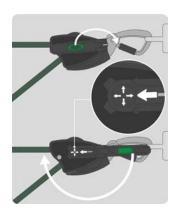
6. Engage the handle and turn until drum slips or until the handle can no longer rotate.
